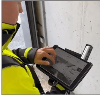
Birdsview: Ground-penetrating radar (GPR) structural assessments
